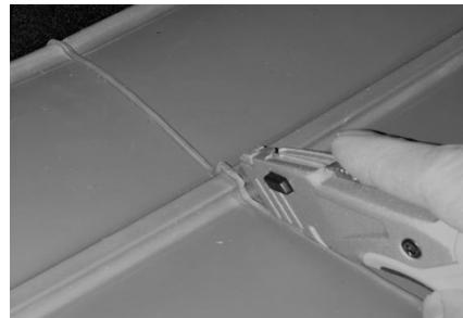
3. Where applicable, feed the strap through the liner that used to lower your third row seats. Vehicles with power folding rear seats will not have the straps.
